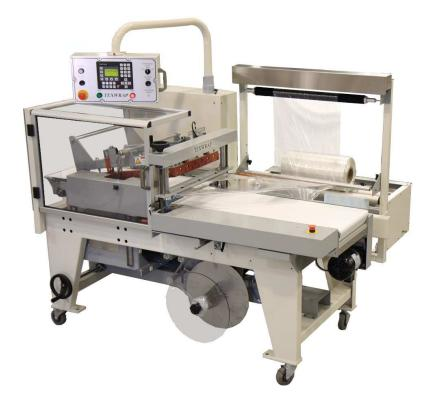
Texwrap's standard line of sealers are designed for L-seal applications where speed and rugged reliability are prime considerations. Built to the same exacting standards as our high speed wrappers, these versatile units are capable of wrapping up to 50 pieces per minute when combined with the proper infeed.
